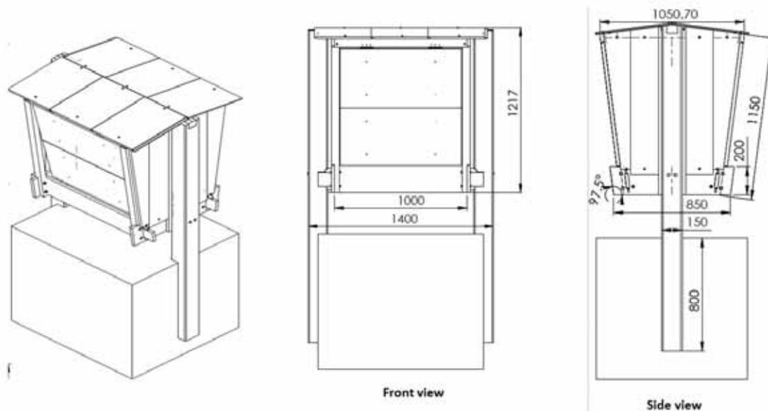
**Image 4** - Concepts, designs, and dimensions – Automatic equipment to supply mineral salt.
