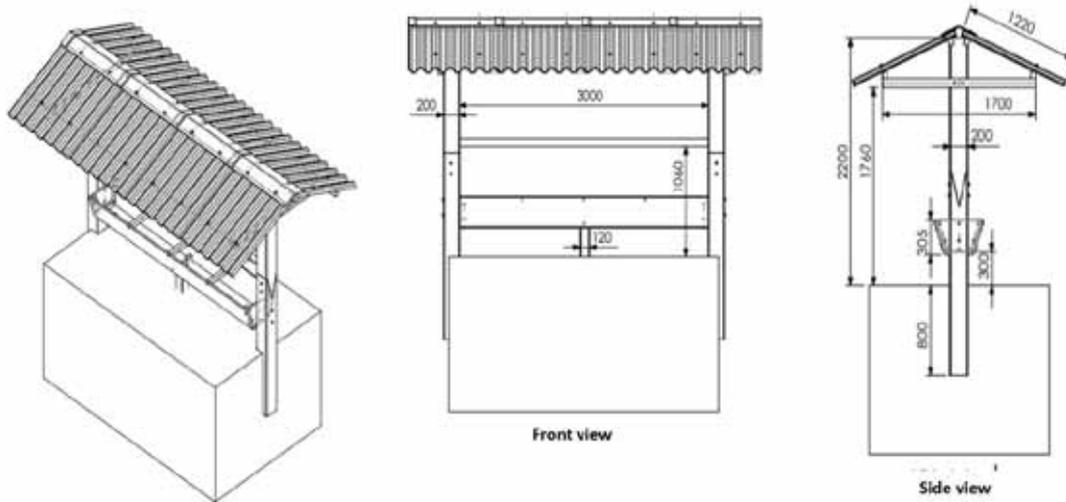
**Image 2** - Concept, design, and dimensions – Stationary trough with cover.
