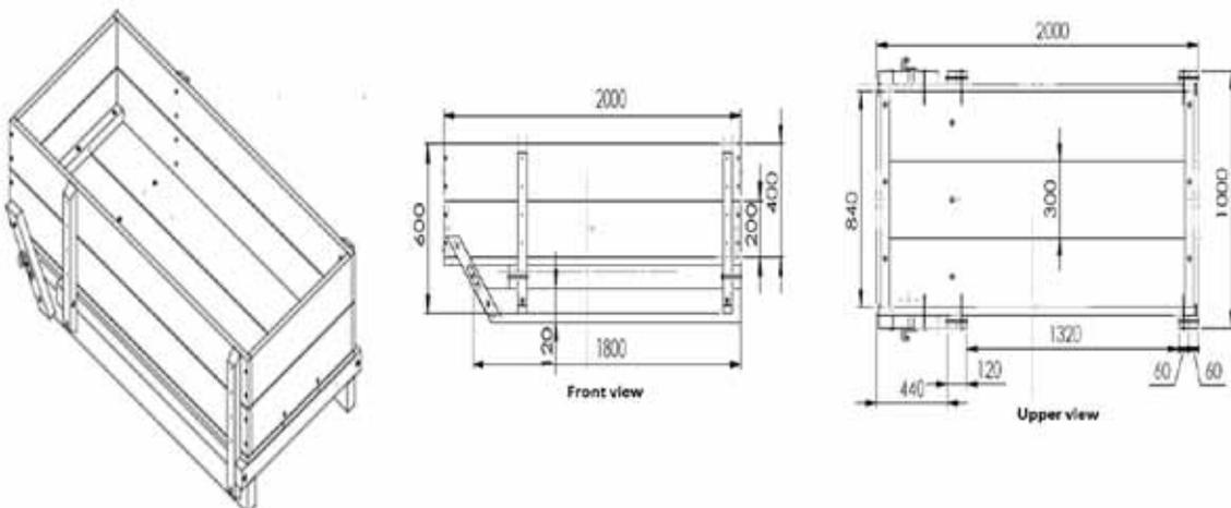
**Image 3.** Concept, designs, and dimensions – Trough-sled without cover.
