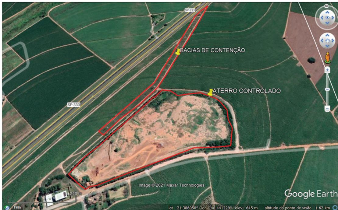
**Figure 3.** The highlight of the main landscape elements in quadrant 3 (larger red outline) represents the controlled landfill in Taquaritinga, SP. In a smaller red outline are the stormwater containment basins.
