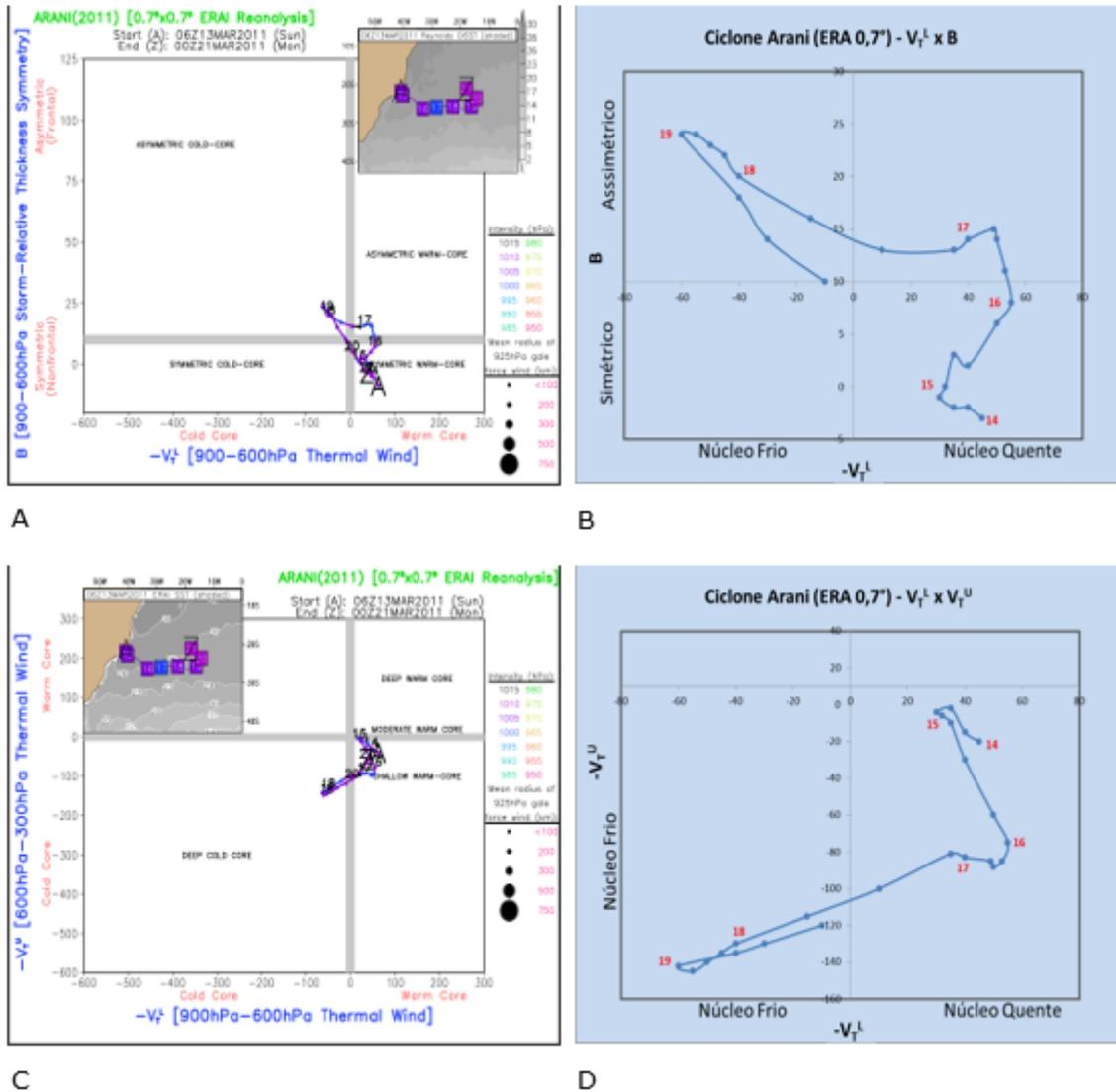
**Figure 7.** Phase diagrams relating parameters B and  $-V_T^L$  (A) and  $-V_T^L$  and  $-V_T^U$  (C), using the ERA-Interim (0.7) reanalysis. (B) and (D) indicate phase diagrams corresponding to the originals (A and C), with scale change. [Source: A and C Florida State University]
