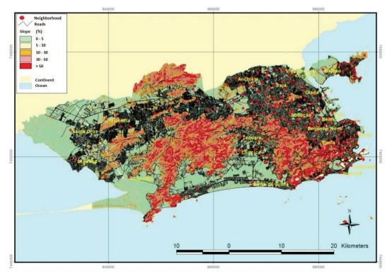
Figure 5. Hypsometric and slope map and its implications for the road and urban design of the city. Source: Prepared by the authors from the cartographic bases of the IBGE (2010).
