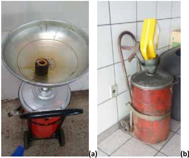
Figure 2. Oil filter and used lubricant packaging through the residual oil draining process.
