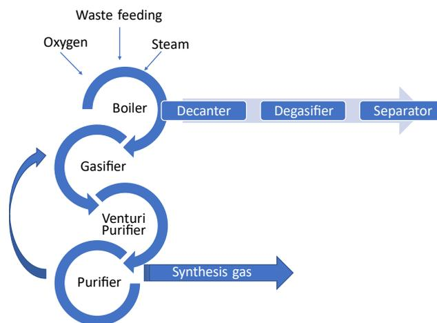
Figure 1. Texaco Gasification Process
