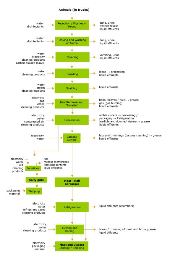
Figure 1. Swine slaughter flowchart Source: Pacheco (2016) food. The stages of pig slaughtering are divided according to the flowchart in figure 1, in which it is possible to verify the stages, from the reception of the animal to the storage and dispatch of the finished product, the points that consume water and the points that generate solid and liquid effluents.
