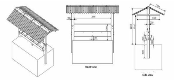
Image 2 - Concept, design, and dimensions – Stationary trough with cover. Source: The authors themselves.
