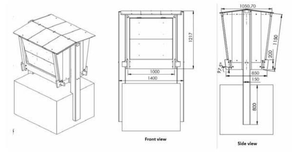
Image 4 - Concepts, designs, and dimensions – Automatic equipment to supply mineral salt. Source: The authors themselves.
