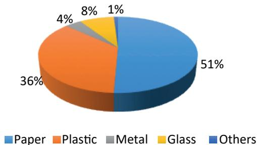
**Figure 2.** Composition of household waste and its recyclable fraction
