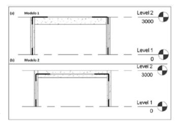
Image 4 - (a) *Revit* standard analytical model; (b) Modified analytical model.
