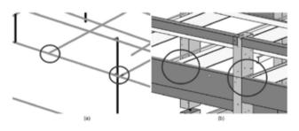
Image 7 - (a) Highlighted connections in analytic model; (b) Connections in the physical model.
