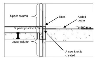
Image 9 - Interpretation *Robot* does when adding a beam some millimeters below a knot.
