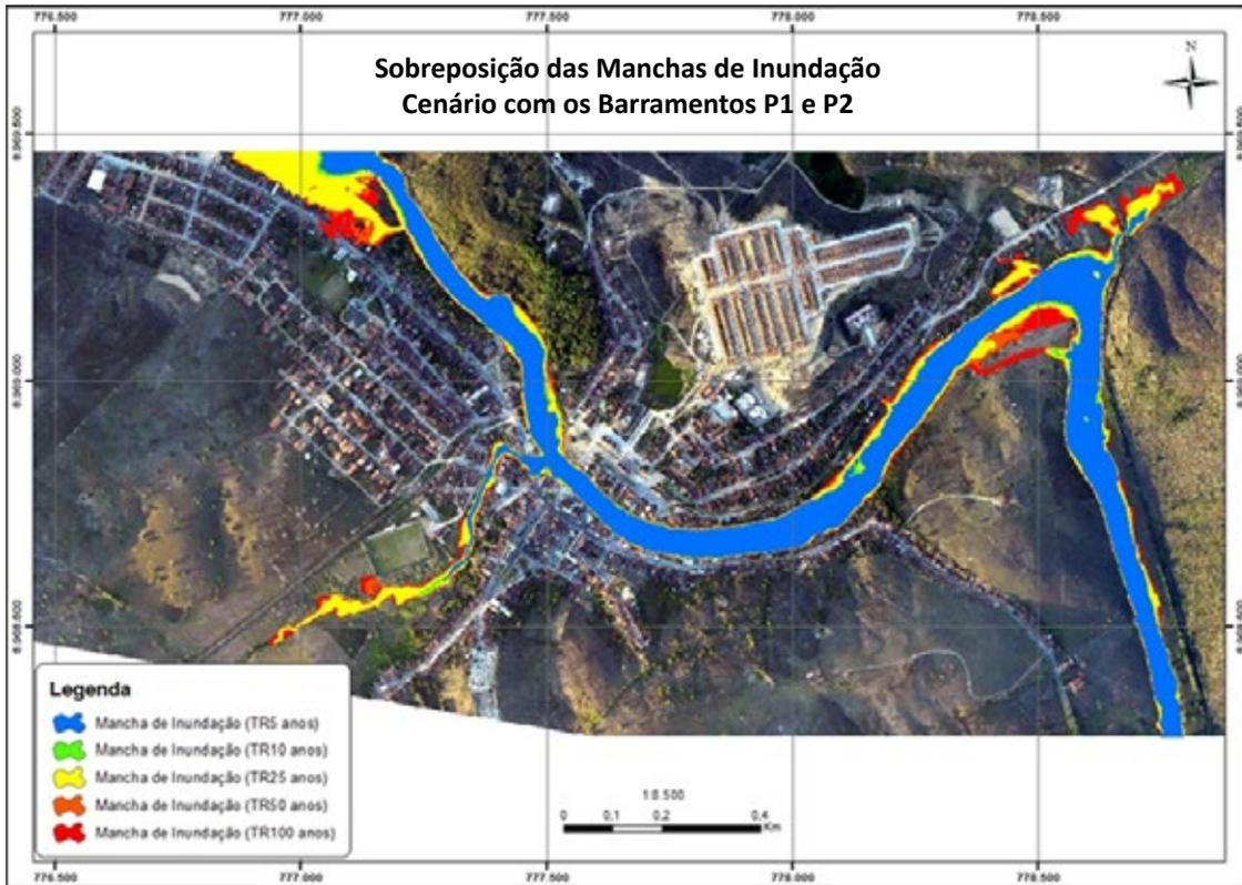
Figure 6. Flood spots for flow rates corresponding to several Recurrence Times, scenario with dams.
